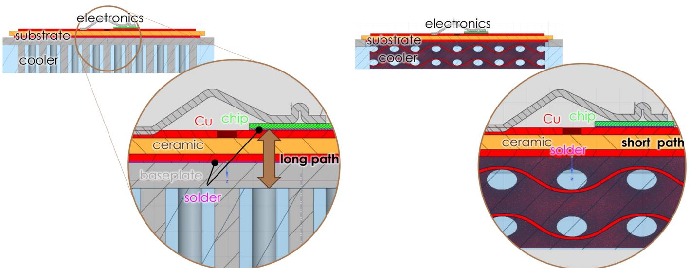
**Fig. 1:** Long cooling path, limited cooling performance, limited geometrical freedom, extended assembly (left). Short cooling path, high cooling performance, geometrical complexity for free, integrated production process (right).
