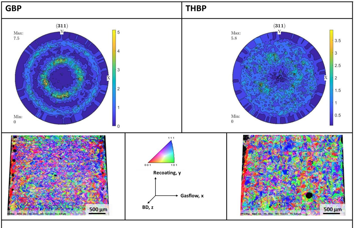
**Fig. 6:** Pole figures (top) and EBSD inverse polefigure maps plotted with respect to building direction (bottom) for GBP (left) and THBP (right). For the GBP specimen, a fibre like intensity distribution is observed, for the THBP specimen, a more homogeneous intensity distribution is observed.
