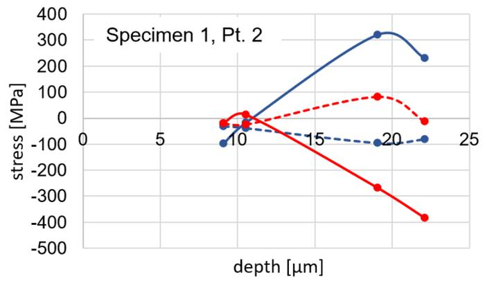
Fig. 7: Example for depth profiles of residual stress in the ceramic layer of a project substrate.
