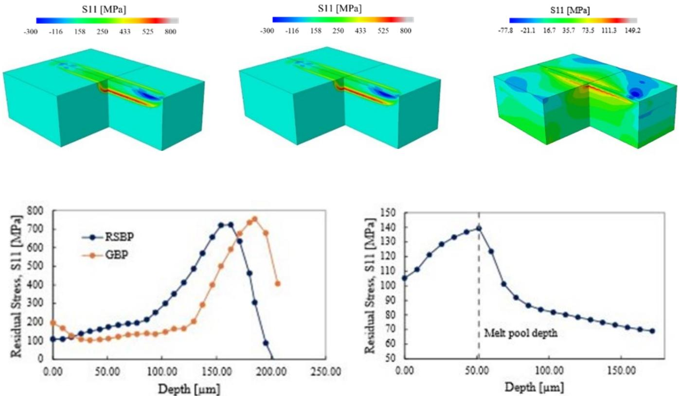
**Fig. 5:** Mechanical stress as determined from the deposition scale model for Ti64, Gauss beam profile (left), Ti64, ring spot beam profile (middle) and pure Cu, Gauss beam profile (right). The top row depicts the stress field, the diagrams in the bottom row the residual stress profile in the centre of the stress field as a function of distance to the surface ("depth").
